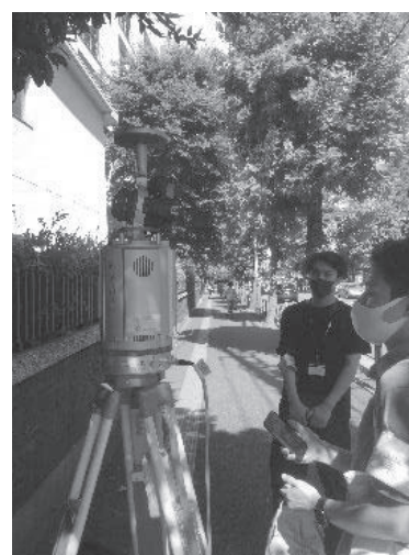
図 3 Terrestrial Laser Scanner (VZ-400i)
